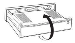
3. Adjusting the viewing angle. Angle should be adjusted slowly without applying unreasonable force.
